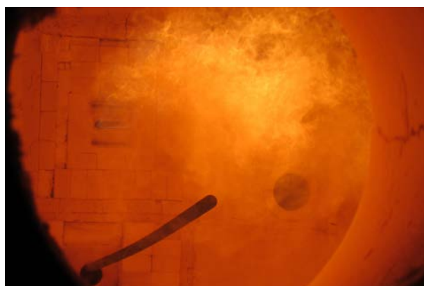
Figure 9: Photo of laboratory measurements of CO concentration below an oxy-fuel flame with over-flame oxygen staging.
