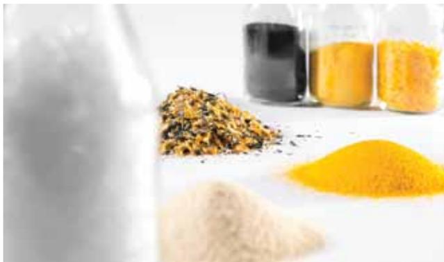
▲ **Figure 2.** Liquid nitrogen is used in certain particle-size-reduction processes to super-refrigerate material, including pigments, plastics, powder coatings, waxes, pharmaceuticals, nutraceuticals, spices, and other food products. Liquid nitrogen makes a material more brittle, allowing it to be easily broken up into small particles using less energy.
