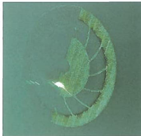
Direct Metal Laser Sintering (DMLS) process using an argon atmosphere to print a prototype.
